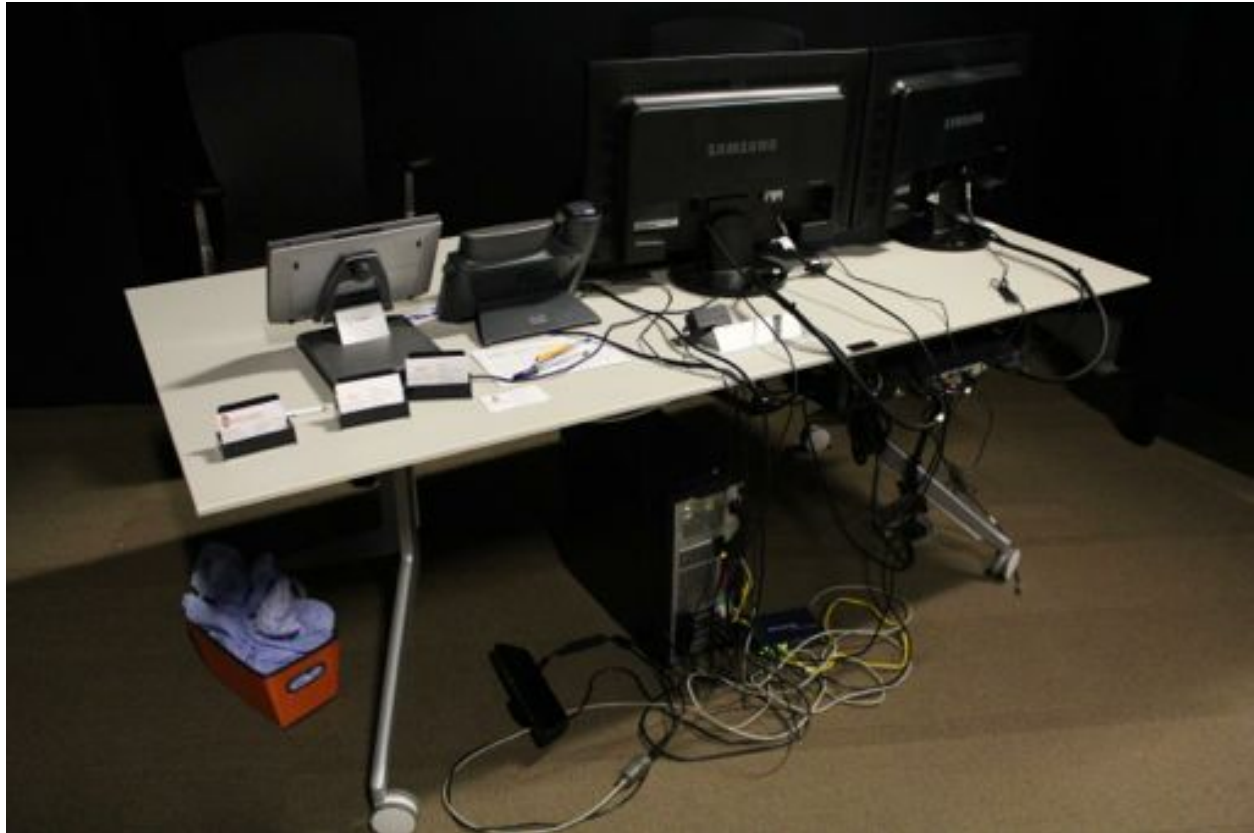
Figure 6 - Additional Machine for peripheral device communication in the CAVE lab space. The head node monitor is shown on the right, while the monitor for the additional machine is on the left. The additional PC is shown underneath the table.
