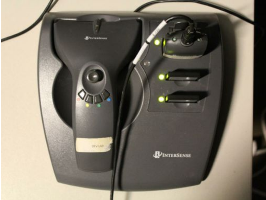
Figure 10 – A charging station for the wand and head tracker, plus extra batteries.
