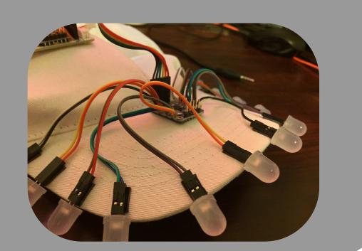
Modern technology available to hobbyists allows us to *sew* circuits into existing garments - this still results in an excess of stitching or bulky electronics plainly visible
